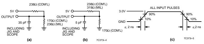
THÉVENIN EQUIVALENT Equivalent to:  $99\Omega$  (COM'L) 2.08V(COM'L) OUTPUT O
